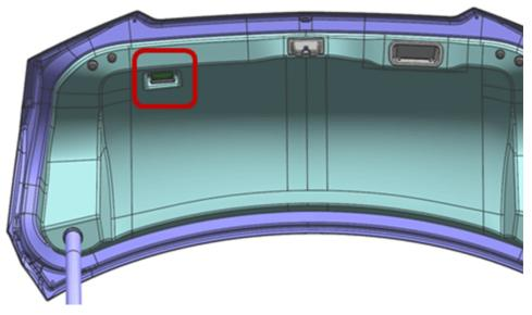
Using the image below as reference check the orientation of the tabs on the bezel. Are the three tabs on the retainer visible or are they obscured by the carpet?
