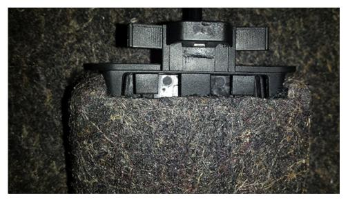
Reinstall liner, ETR and bezel and confirm smooth operation.
