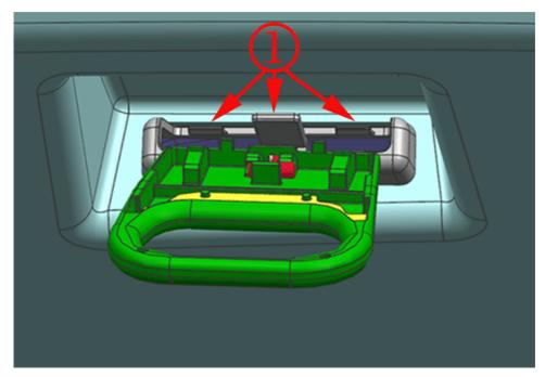
Interference from the trim can cause the handle and cable to bind. Any sort of preload on the ETR cable will not allow the latch to release when any of the electric switches are used.
