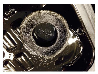
The amount of debris shown in this picture would not be considered normal and the transmission should be replaced.
