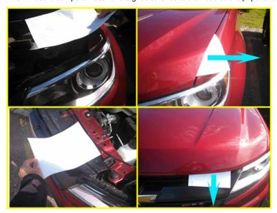
If bumpers and latch are not in adjustment based on the paper test in Step 2, continue with steps 3-5.
