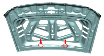
Inject foam into the second hole from the side
