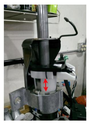
2. The upper intermediate steering shaft to lower column shaft bolt and nut (2) may be contacting the inhibitor/shiftier cable bracket, as shown below.
