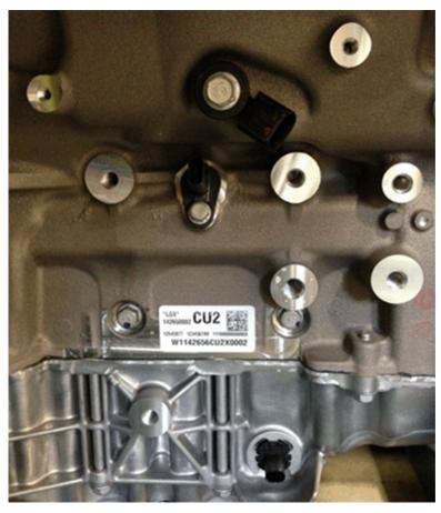
As shown in the above photos, the engine broadcast code can be found on the front engine timing chain cover beneath the bank 2 exhaust camshaft location or the bank 1 location just beneath the crankshaft sensor.
