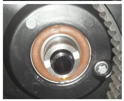
**Note:** When removal of the actuator is required, insure installation of these sleeve's during the reassembly of the engine. These sleeves are not shown in the parts imager and are only available as part of the camshaft actuator assembly.
