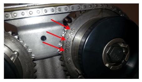
The camshafts can be identified by the last four digits of the part number located on a machined surface between the number 2 and number 3 cylinder camshaft lobes.
