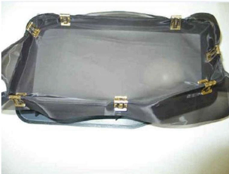
5. Reinstall plenum cover cap, insure cover is flat and free of damage, using Kent air dry sealer or RTV around the perimeter of the plenum cover cap. Allow sealer to dry following manufactures recommendations.
