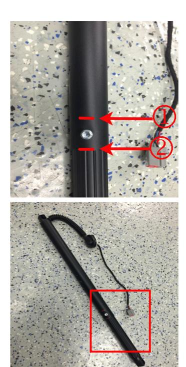
Note: The screw will hold the actuator together for removal.
