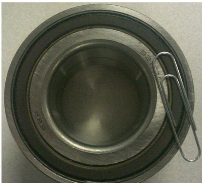
The picture below shows the opposite side of the wheel bearing for reference. This side would be facing outboard, away from the wheel speed sensor.
