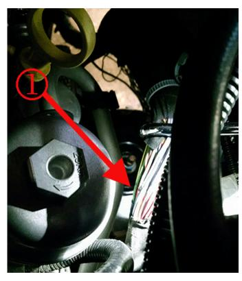
If you encounter either of these scenarios, inspect, repair (as necessary) and route the engine harness away from these possible contact points.
