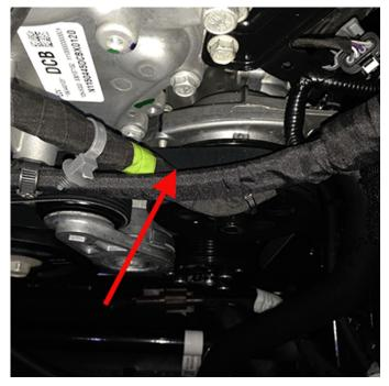
Wiring chafing on the oil filter housing:
