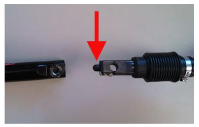
3. If not present in the upper I-Shaft, check down the inside of the lower I-Shaft and joint for the plug. Invert the shaft and tap the open end on a shop towe on a workbench. If found, remove the plug, discard and reinstall the lower shaft.
