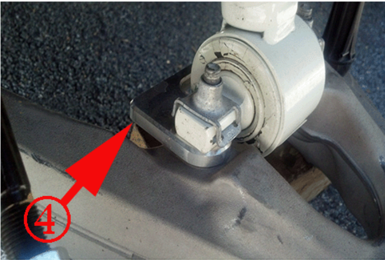
4. Aftermarket lift kit blocks installed
