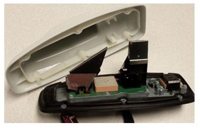
**Important:** The painted antenna cover is not intended to be removed. Do Not remove the antenna cover as this may compromise the sealing performance. Do Not reuse the original antenna painted plastic cover, there is a potential quality concern with the cover. Latest service parts include updated covers.
