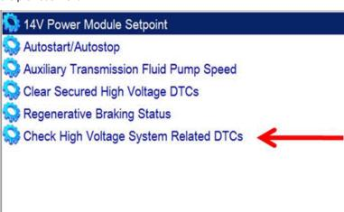
3. Now select clear the High Voltage DTCs in the HPCM and hit the reset button on the bottom of the screen. Wait 45 seconds before exiting the screen
