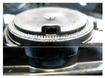
If the PCV orifice external port is leaking oil or vacuum, replace the camshaft cover assembly.
