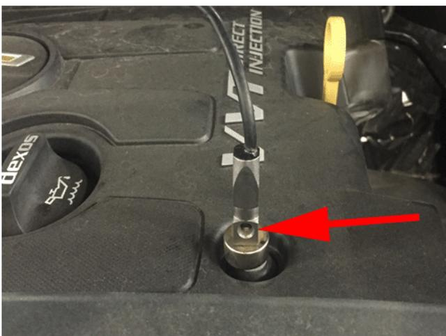
2. Using a Pico Oscilloscope Diagnostic Kit, mount the PicoScope single-axis or 3 axis vibration sensor (TA143) on the intake cover bolt with the hole on the sensor facing in the forward direction as illustrated above.
