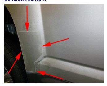
Some customers or dealership personnel may comment that the paint protection patch is missing from the rear door as shown in the illustration above. Recently a change was made that removed the protection patch from production.
