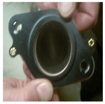
Note: When installing the turbo outlet gasket, make sure to position on the studs correctly as shown in the illustration above.
