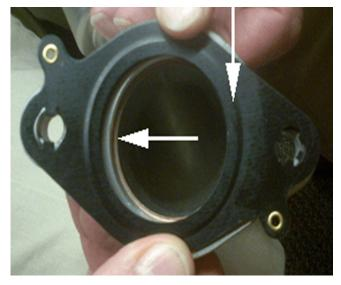
Note: If the gasket is flipped, as shown in the illustration above, it will reduce the outlet flow.
