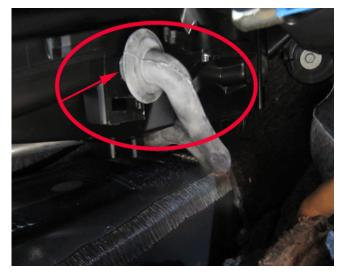
Note: Shown in the illustration above is where the plant temporary installs the A/C hose during Instrument panel installment. Do not drill out the
