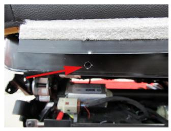
**15.** Drill two 1/4 in. holes in the steel seat support at the marked location as shown.
