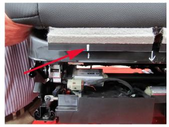
Mark the same two locations on the corresponding seat cover mounting "J" channel.
