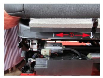
13. Measure 100 mm (4.0 in) on both sides of the center mark and mark the two locations with a paint pen (1).
