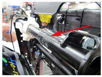
4. Using a small brush, apply GM Super Lube GM P/N 12371287 (In Canada, use 10953437) as shown. Ensure the complete contact surface is coated.
