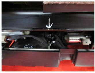
**12.** Find the approximate center of the front seat steel support and mark the location with a paint pen.
