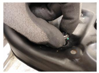
7. Hand start the four screws; Do NOT tighten.
