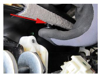
21. Insert two (5/16" stem diameter; 5/8" stem length) push pin retainers, GMP/N 00332364 or the equivalent, into the drilled holes from the underside as shown.
