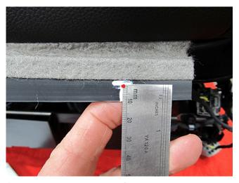
16. On the two seat cover mounting "J" channels, measure up 10 mm (0.39 in) from the lower edge and mark the location.
