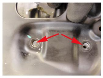
**6.** Align the holes in the seat pan with the holes in the pivot blocks.
