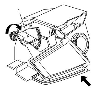
**5.2.** From the back side of the housing, rotate the damper gear so the U-shaped guide aligns with the pivot pin on the back side of the inner ashtray/bin.
