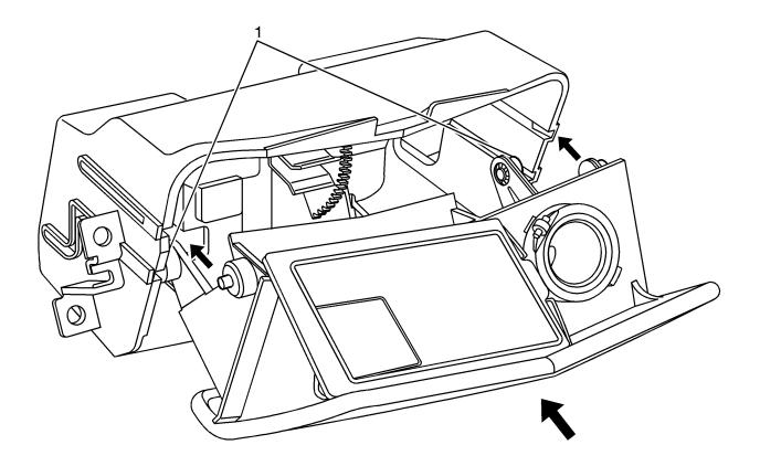
5.1. Start by sliding the two lower metal pivot pins (1) on the ashtray/bin door into the track guides inside the housing. Then slide the upper two metal pins into the housing.
