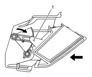
5.3. Push on the door to engage the pivot pin onto the damper gear guide while moving the door rearward.
