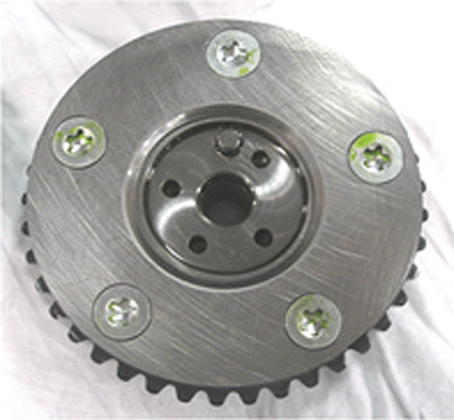
4 screw design uses P/N 12632859 thrust washer
