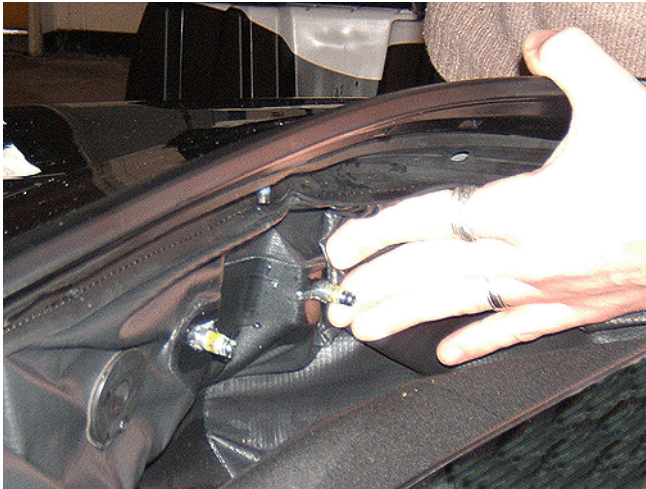
6.4. Push the pleats toward the trunk, then pull the pleats and bag material taut, and position the folds next to the outboard bracket stud.
