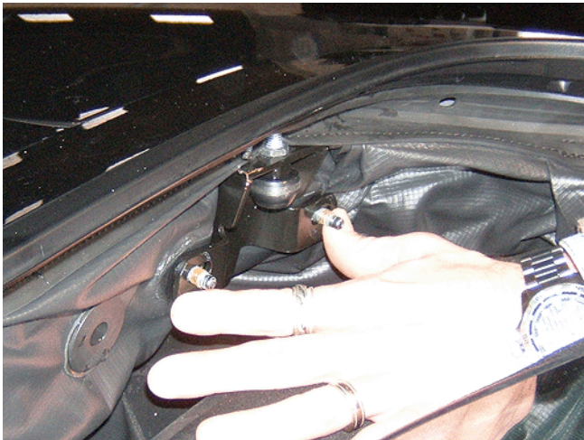
6.5. Reinstall the stowage compartment bracket(s), capturing the folds beneath the bracket, and tighten the nuts.
