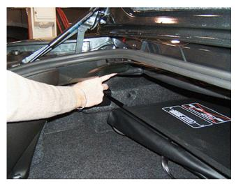
Open the trunk and access the water management bag in the rear compartment. The low points of the bag will be on the left and right sides of the
