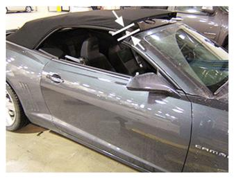
3. Carefully start to lower the convertible top and stop movement when the top is approximately 100mm (4 in) from the windshield header.
