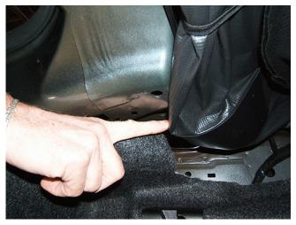
2. Squeeze the lowest locations of the water management bag (left side shown in the graphic above) listening and feeling for any indication of ice. If ice is present, DO NOT lower the convertible top until the ice has melted.
