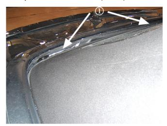
4. Inspect both sides of the water management bag for possible ice formation in the areas below the rear glass (1). If any ice is present, DO NOT lower the top any farther until the ice has melted.
