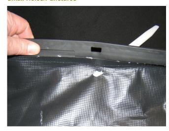
For smaller repair areas, apply \*Kent Automotive Quick Seal™ Seam Sealer Black P/N P10556, or equivalent, directly to the bag material:
