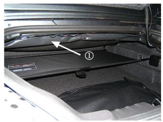
After water testing and visual inspection, the technician may find that the convertible top water management bag (1) is leaking due to a puncture or tear in the material. Aside from obvious holes/tears, the following locations should be closely inspected as potential leak areas:
