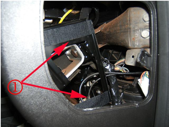
Install the other side of the 2" Velcro® 191195 Reclosable Loop Fastener Tape (hook and loop) or equivalent to the OnStar® module bracket as illustrated. Use the Reclosable Loop Fastener Tape or equivalent to secure the OnStar® module to the bracket.
