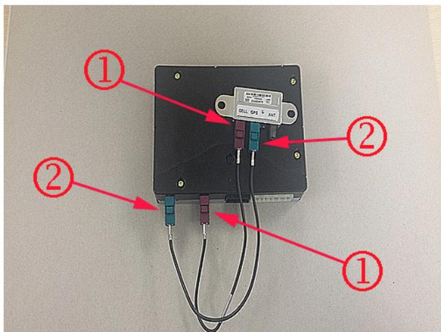
4. Connect the male to male cable (P/N 23310710 ) to the cellular connector (1) to the splitter as shown above.
