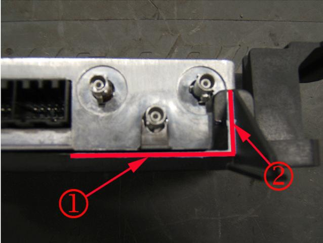
Remove only enough material from the lower edge (1) and shoulder (2) from the bracket to allow the module to seat fully.
