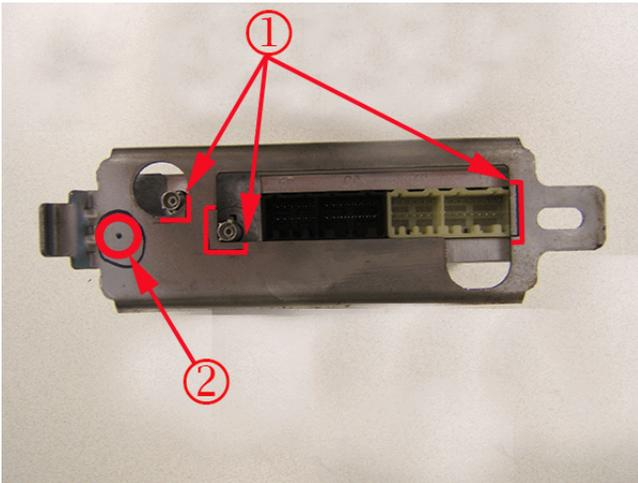
After the original module is removed.
