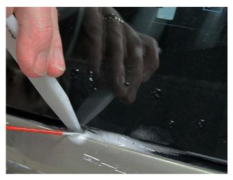
2. Using the spray nozzle attachment, insert the nozzle in the area between the molding and the body and apply a liberal amount of GM Super Lube, P/N 12346241 (in Canada, use 10953474).
