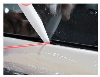
1. Using a plastic trim stick, lift the windshield molding away from the windshield opening exterior surface.
