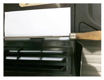
Detach the storage compartment door from the body side trim panel, and using a file or similar tool, remove 1.0 mm (0.04 in) of material from the storage door latch.
