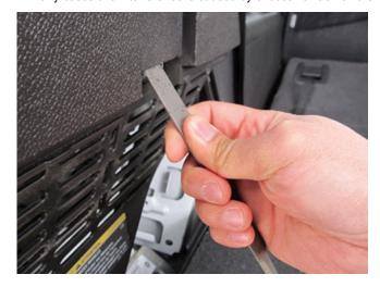
Remove the storage compartment door and inspect the side trim panel opening for flash. If flash is present, it should be removed with a file inserted at a steep angle.
