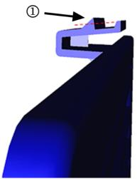
Once the flash is removed, re-install the storage compartment door. If it latches easily, no further action is required. However, if it is still difficult to latch, it may be necessary to remove approximately 1.0 mm (0.04 in) of material from the pointed edge (1) of the jack storage compartment door latch.
