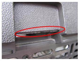
**Note:** The excessive flash may be folded back behind the panel and difficult to see, but it can still be detected by feeling the back side of the trim panel opening. In many cases this interference is caused by excessive flash on the inside edge of the body side trim panel opening, preventing proper engagement of the latch
