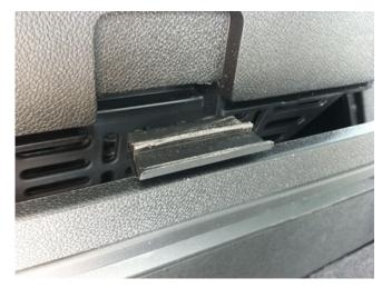
Reinstall the storage compartment door and verify improved function of door latch.
