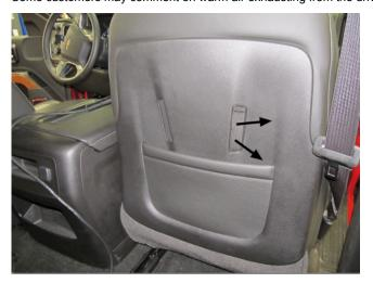
The cause of this condition may be that during cooled seat operation, a direct flow of warm air exhausts from the upper seat back ventilation heating/cooling blower.
