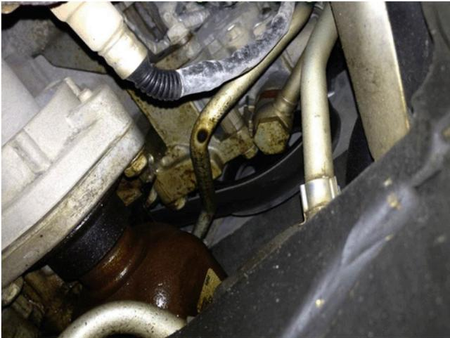
This is also a leak because there is a droplet formed on the bottom of the power steering line and fluid has dampened the drive axle.
