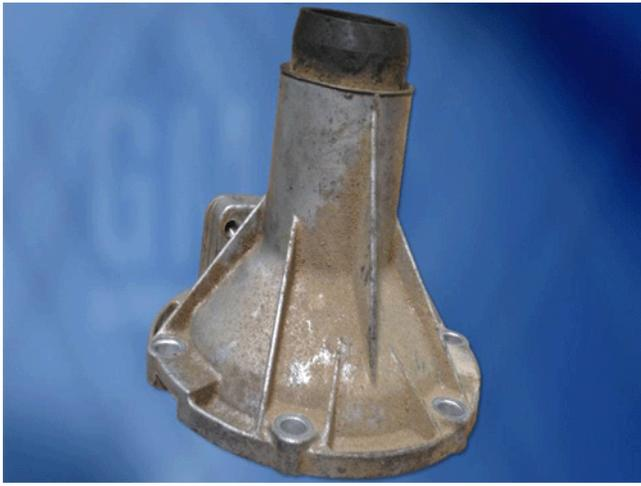
The housing illustrated above just has a light coating of dirt; there is no sign of fluid. So this would also be considered seepage. A very small amount of fluid coated the outer surface of the housing and dirt was attracted to the moisture.
