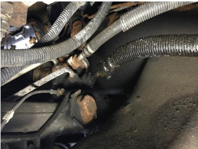
This would also be considered a leak because fluid has coated the fitting and hose. Although there were no droplets hanging from the component, it's obvious that a reasonable volume of fluid has been lost and when we followed the line to its low point, we did find droplets there.
