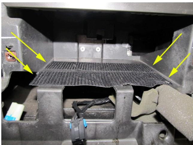
3. In the open space in the instrument panel (I/P), where the original module was, install on the bottom portion of I/P the other side of the 2" Velcro® 191195 Reclosable Loop Fastener Tape (hook and loop) or equivalent as shown above.
