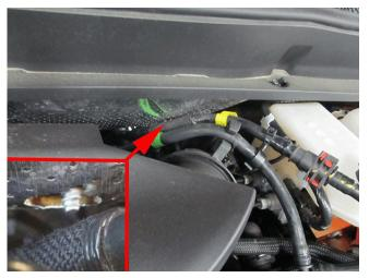
If this condition exists at the contact point illustrated above, re-routing and securing of the vacuum lines with a nylon tie strap should be performed. Follow the instructions listed below:
