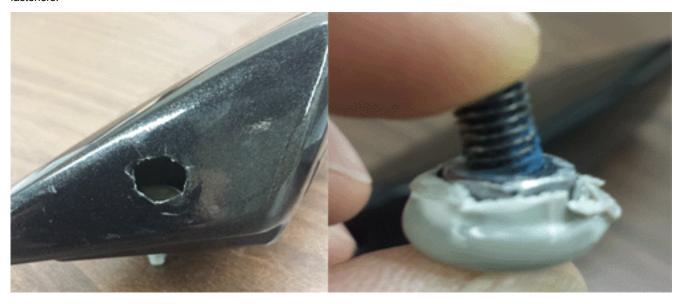
The use of power tools should not be used due to the fact that this could lead to damage to the fasteners and/or the spoiler.
