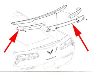
During the installation of the rear wicker bills that are fastened on the rear spoiler, some technicians may revert to the use of power tools to tighten the fasteners.
