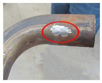
6. Using a cut off wheel, remove the exhaust alignment button off the catalytic converter.
