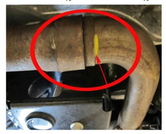
**Important:** Mark the location on the exhaust where the exhaust goes into the catalytic converter.
