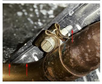
This may be due to the stainless steel alignment button on the catalytic converter, causing the exhaust to come in contact with the heat shield from not being positioned correctly.
