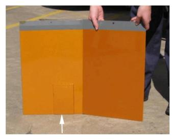
This photograph shows the same paint test panel with a slight crease in the center, creating an angle in the panel similar to the Camaro door to quarter panel relationship. The finish on the right side of the panel has "shifted," creating a different hue of the same color. Note the arrow shows the paint standard on the left side of the paint test panel in the same position as the first photograph.
