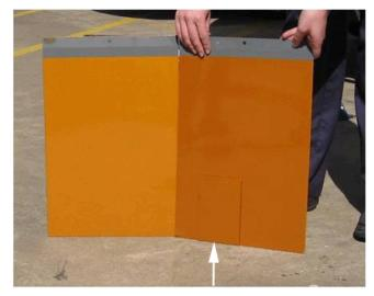
This final photograph shows the same paint test panel described in the second photograph. In this photograph, the arrow points to the same paint "standard" used in the first two photographs but it has been repositioned to the right side of the paint test panel. Note the paint "standard" has shifted along with the finish on the paint test panel.
