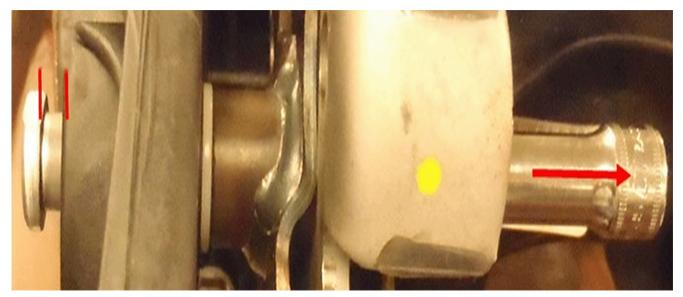
4. Insert the new pivot pin in the hole and push until the socket is out and the head of the pivot pin is 10 mm from being seated.
