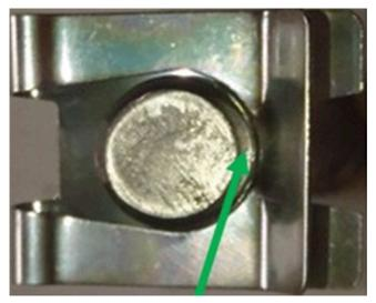
**Note:** Ensure that the retaining clip is completely engaged over the new pivot pin.
