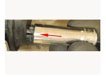
2. Using an 8 mm socket, push against the ramps of the fingers locks and continue inserting the socket into the hole until the pivot pin is pushed out and discard.
