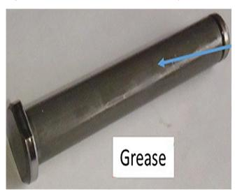
3. Apply a thin coating of GM Super Lube, P/N 12346241 (in Canada, P/N 10953474) or equivalent, on the entire length of the new pivot pin.
