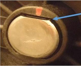
5. Align the flats on the pivot pin with the flats on the housing boss, then push the pivot pin inward until fully seated.
