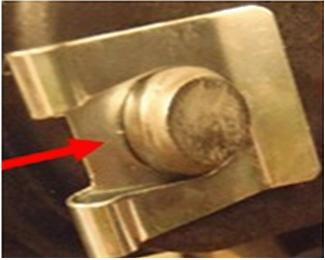
**6.** Insert the two fingers on the retaining clip into the groove on the new pivot pin and push until fully seated.
