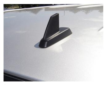
Grasp and physically inspect the XM, cellular mobile phone, and/or OnStar® antenna for looseness and/or damage. If the antenna is mounted securely and exhibits no signs of physical damage, follow regular diagnostic information in SI to address any customer concern.
