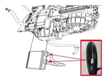
If this condition exists, replace the inlet and outlet heater core pipes and O-rings. Use the Heater Core Replacement procedure in SI. For the Spark EV, refer to the Heater Inlet And Outlet Pipe Replacement in SI.
