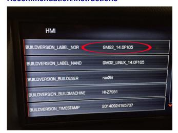
Before updating software, check the HMI build version. The HMI build version label should be earlier than GMG2\_14.0F105.
