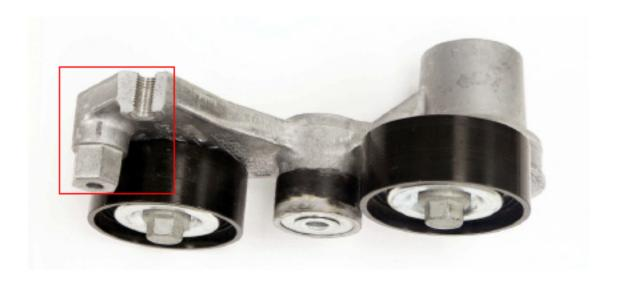
If you encounter a vehicle with the above concern, inspect the MGU belt and tensioner. If the belt looks like it was cleanly snapped or if the tensioner is broken at the attachment boss (shown above), contact the engineer listed below for further instructions.
