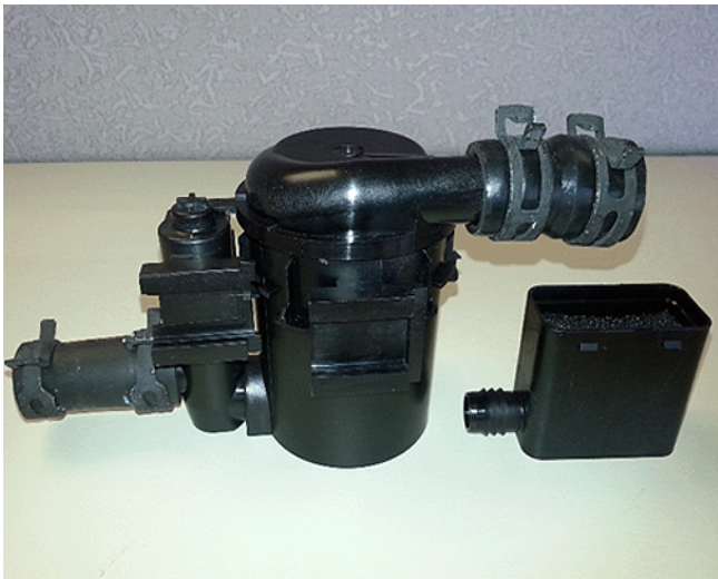
Revised design EVAP CVS valve shown above.
