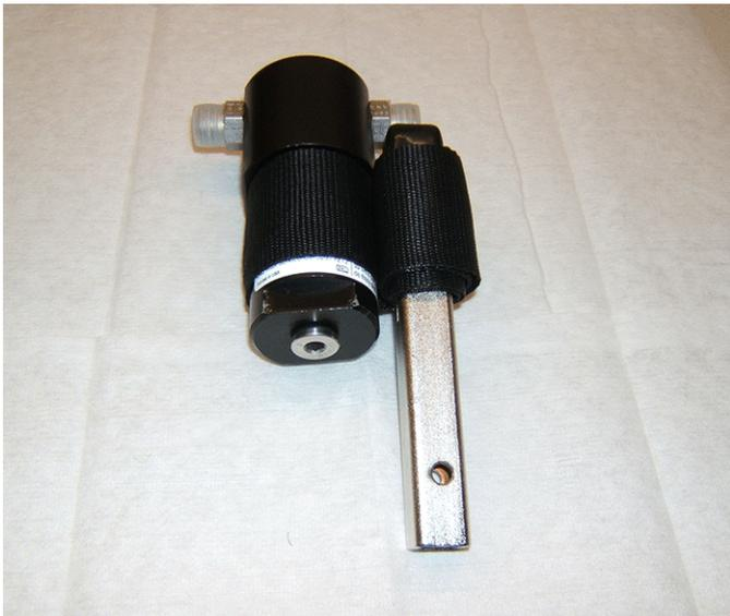
Due to the limited access, the recommended tool to remove and replace the CNG high pressure fuel filter housing/element is a strap wrench or a crowfoot wrench.
