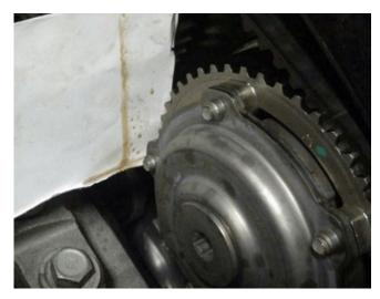
It may require you hold the paper near each sprocket to identify which sprocket is leaking. The oil shown on the paper in the picture is after approximately 30 seconds of operation at 2000 RPM. The arrows indicate the area of the potential leak.
