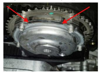
Clean any residual oil from the camshaft sprockets. Using white paper, run the engine off idle at 2000 RPM to check for oil being ejected from either the intake or exhaust camshaft sprocket.
