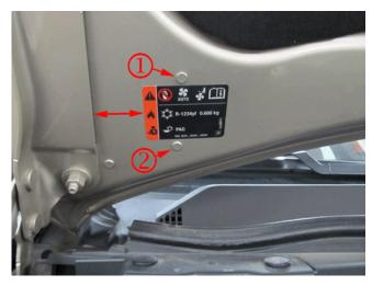
Install the label  $1\frac{1}{2}$  inches (38 mm) parallel to the right hood hinge in between the two rivets like shown above.
