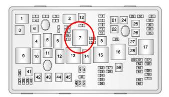
If no other root cause is identified through normal diagnosis, replace the KR75 Engine Controls Ignition Relay (shown above) with the updated relay, P/N 13595908.
