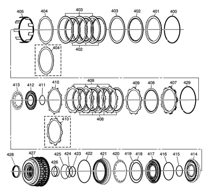
**Important:** When reassembling these clutches, the retaining rings (400 and 429) must be properly aligned in the housing. Align the retaining ring gap with the missing snap ring groove punch in the housing or the offset punch in the housing. Failure to do so may cause damage to the clutch assembly.
