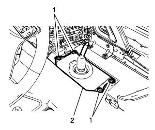
11. Install the lower transmission control closeout boot (2).
