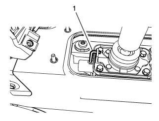
$\textbf{10.} \ \ \text{Lift to release the shift control neutral lock pin (1)}.$
