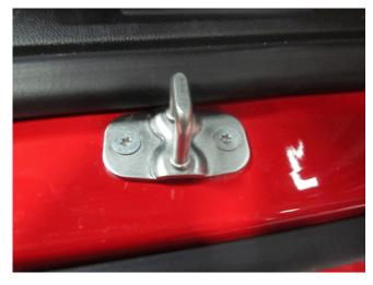
This condition may be caused by the rear door lower striker being out of position.
