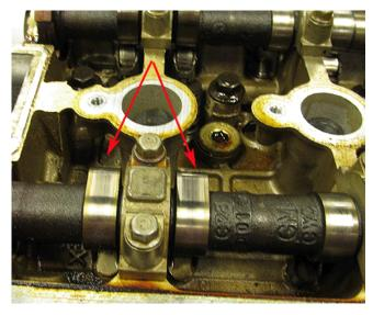
• Camshafts and roller follower will have wear markings. This is normal and do not need to be replaced (refer to picture above).
